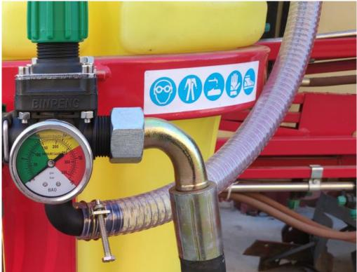
5. The filter cup is fixed at the bottom of the frame, and the elbow on filter cup and the elbow on pump is connected with the transparent
