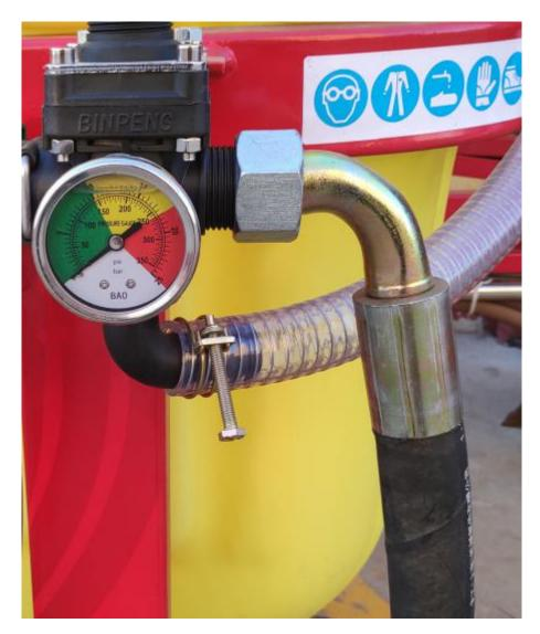
8. Adjust the pressure, the pressure should not exceed the red display area, otherwise the machine will be damaged if the pressure is too high.
