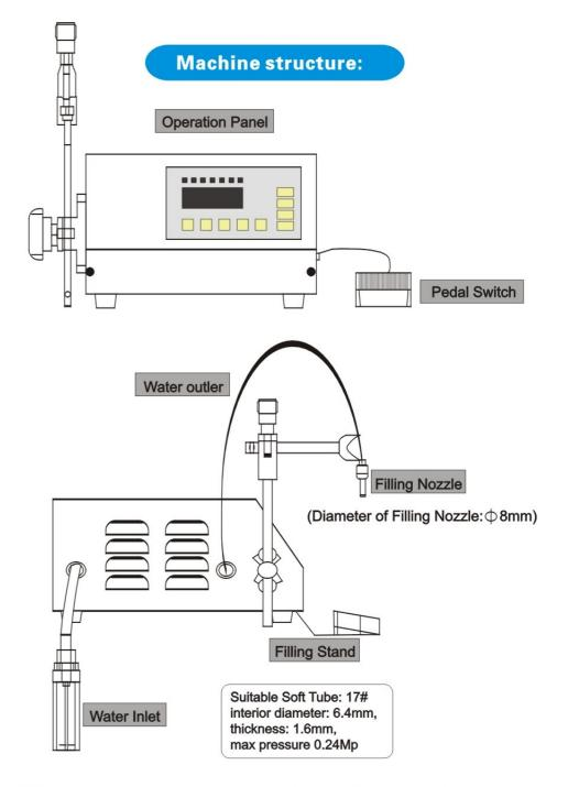
Different liquid needs to choose different material of tube. The tube provided by us is silicone tube.
