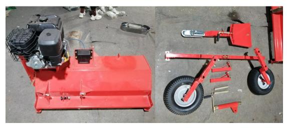
(1)1pcs main body (2)2pcs wheel shaft assembly (3)1pcs Crossbeam weldment (4)2pcs springs (5)1pcs adjust handle weldment (6)2pcs protective tube weldment (7)1pcs tow bar assembly
