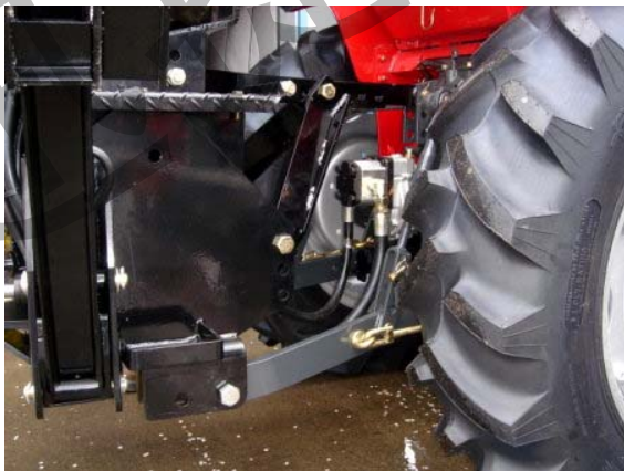
3 Point Shown Mounted on a Mahindra Tractor
