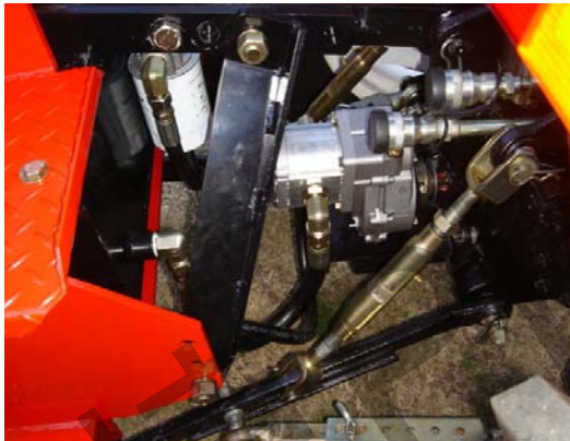
Shown with optional PTO pump and reservoir.
